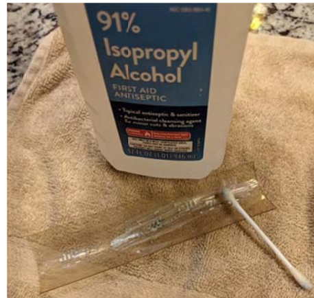
2. Cleaning an original plastic dial face with a Q-tip and 91% rubbing alcohol.
