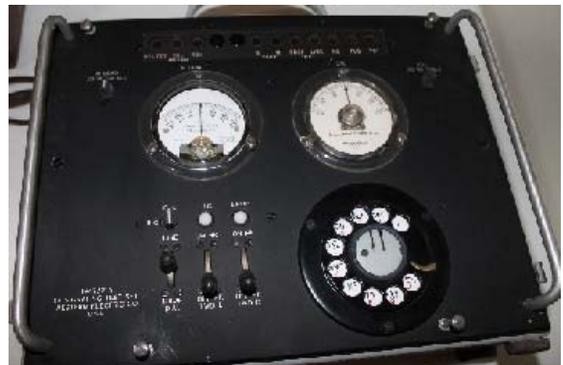
**Western Electric model 1A Signal Test Set used in the telephone industry.**
