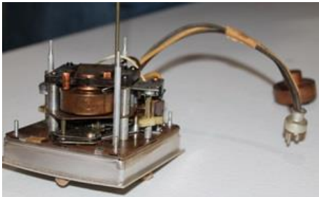
A Telechron clock motor. The brass disk behind the power connector is an H3 rotor.
