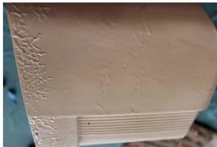
Side of radio showing paint bubbling.
