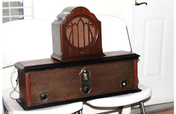
Above is the fully-restored Graybar Model 310 early AC set from 1928 that is the main prize for the Fall Swap Meet Raffle. It is a fairly uncommon set using a Radiola 18 chassis and is paired with a nice original-finish Bremer Tully cathedral-shaped speaker.
