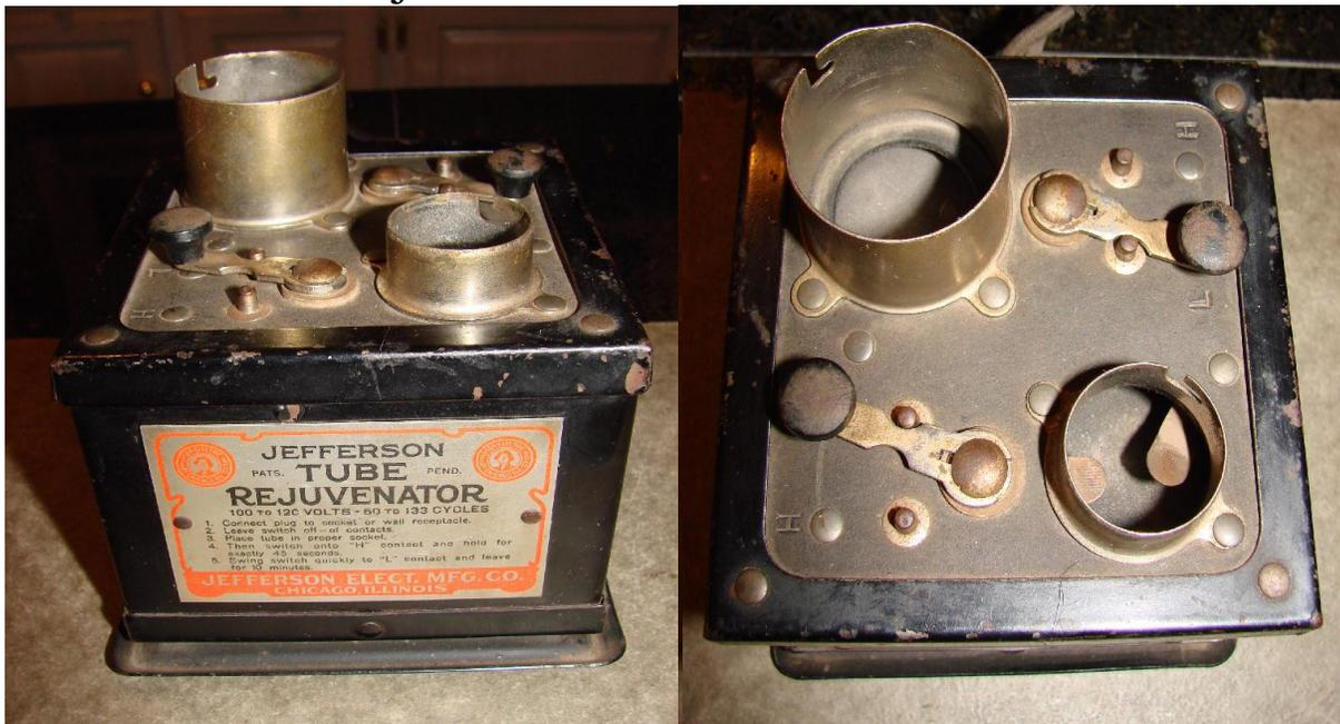
This month's featured item is the Jefferson Tube Rejuvenator. It was made in Chicago by the Jefferson Electric Manufacturing Co. These were made from the mid 1920's probably up until the early 1930's. This is the most common of the tube rejuvenators made. The black paint of the body is not heavy, so it is hard to find one in good condition. The one pictured above is the one I use.
